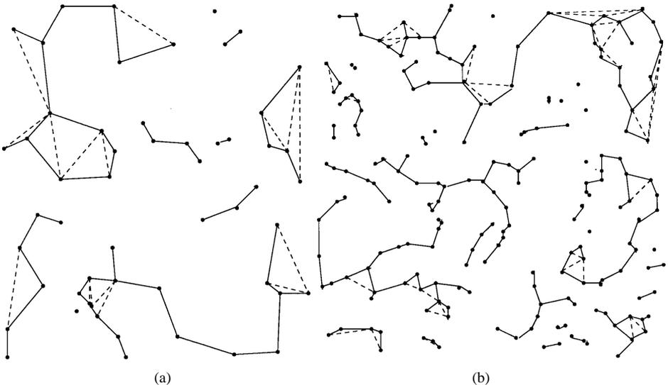
Figure 8. Some example of experiment, where part (a) has 55 points and part (b) has 200 points. The solid lines are  $\beta$ -skeleton and dashed lines are new edges by our method.
