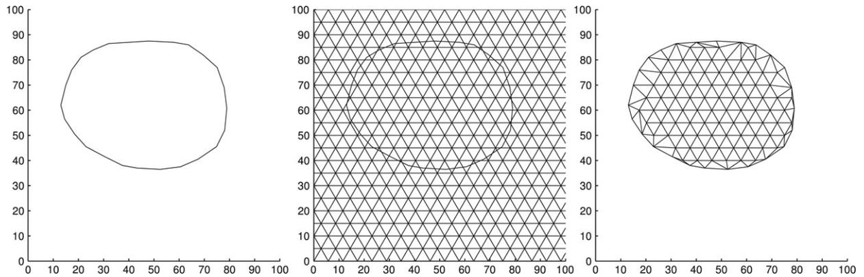
Fig. 6. Experimental results: The left illustration denotes the initial polygon, the middle illustration denotes the initial polygon with the equilateral triangle lattice with edge length  $l$  and the right illustration denotes the obtained triangular mesh with  $\beta = \frac{1}{2}$  after running our algorithm.
